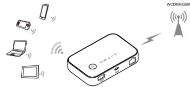
**Ethernet port connection (LAN) :** Connect your Mobile WiFi to a computer using a network cable.
